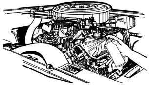
Rinse with a mild stream of water. Collect run-off with plastic sheet placed under the motor. Idle engine to dry.
